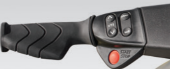
HIGH-PERFORMANCE VTS™ (VARIABLE TRIM SYSTEM)
